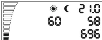
You see the alternate blinking of sun and moon segments. Enter SET/SAVE to change the switch level value between day and night time. The lower the value, as less light it needs to change from day to night time mode.
