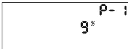
Now you can set the speed which should correspond to 1% of the minimum speed. Push the knob to change the displayed value with rotating the knob. Save the new value with pushing the knob. Turn clockwise the knob and go to the next setting. Repeat for all coming settings.
