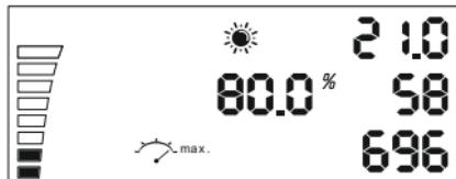
Minimum speed setting day time. Here you can choose the minimum speed of the ventilator which never should be undercut. On the down left side speed bar you can see the actual setting for each filled segment is 10% fan speed. Change the settings again with SET/SAVE as described above.
