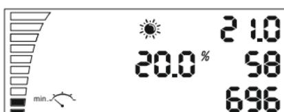
For example: 10%rh at 60% humidity the fan starts to work at 60% humidity and +10%rh at 70%rh it reaches its maximum speed.
