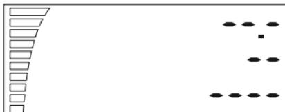
Next it starts initializing the sensor and in case this screen stays at this stage, there is a fault with the sensor or the communication itself. Check the connection from the sensor to the device. If it is still faulty return the device to be repaired.
