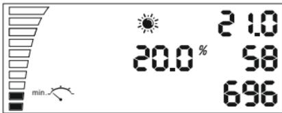
Minimum speed setting day time. Here you can choose the minimum speed of the ventilator which never should be undercut.
