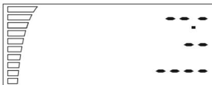
Next it starts initializing the sensor and in case this screen stays at this stage, there is a mistake with the sensor or the communication itself. You have to return the fan for repair.
