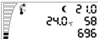
This last setting is the switch over time between day and night mode. This is used to avoid an immediate switching between day and night mode. If the light sensor reaches the switching level a count down starts according to the value in seconds you are entering here.
