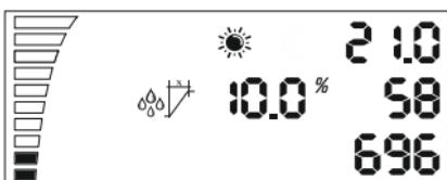
Hysteresis setting for the humidity day time, as described above the hysteresis for temperature you can change here the controlling range for the humidity value. For example: 10%rh at 60% humidity the fan starts to work at 60% humidity and +10%rh at 70%rh it reaches its maximum speed.
