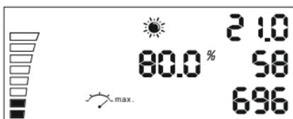
You see the alternate blinking of sun and moon segments. Enter SET/SAVE to change the switch level value between day and night time. The lower the value, as less light it needs to change from day to night time mode.
