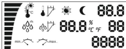
The power LED blinks and the fan starts to initialize. This takes a few seconds. As first you will see a screen with all the LCD segments and back-light working.
